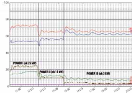
The controller selects an appropriate dose of fuel and air to reach the required thermal power. The chart presents the courses of three sample powers, depending on energy reception.
